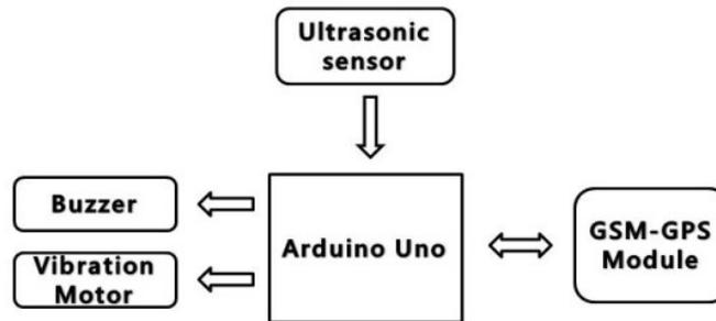
Figure 2. Function of Smart Cane
