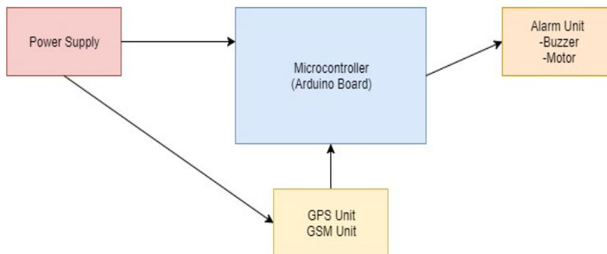
Figure 1. System Architecture
