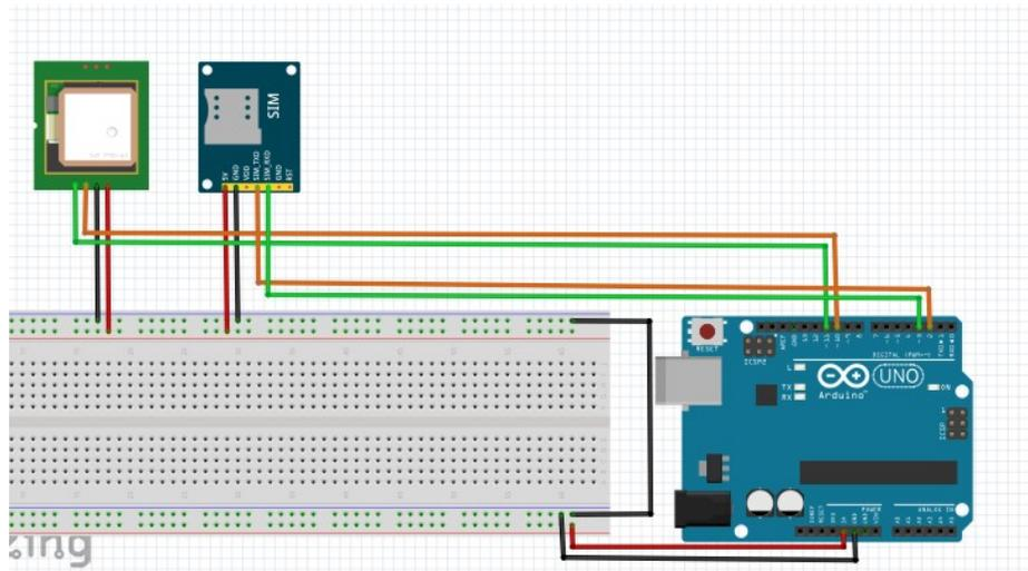
Figure 4. GPS-GSM Module
