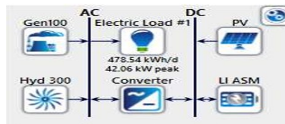
Figure 4. HOMER System Architecture [18]
