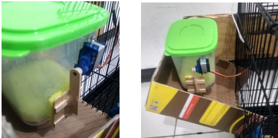
Figure 6. Installation of Bird Feeding Valve
