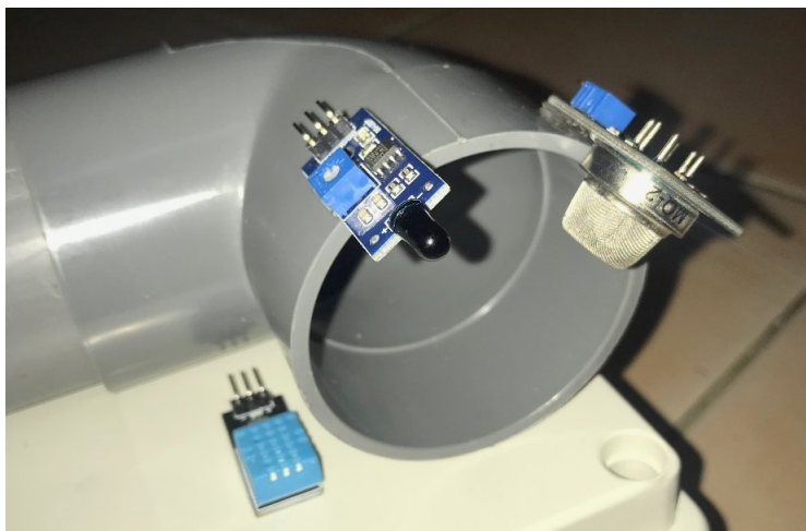
Figure 4. Sensors on pipeline
