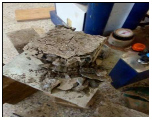
Figure 9. Concrete Specimen: Failed Rubberized Concrete Cube
