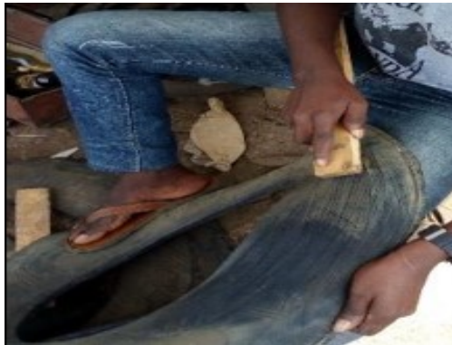
(c) Scrubbing the Rubber Surface
