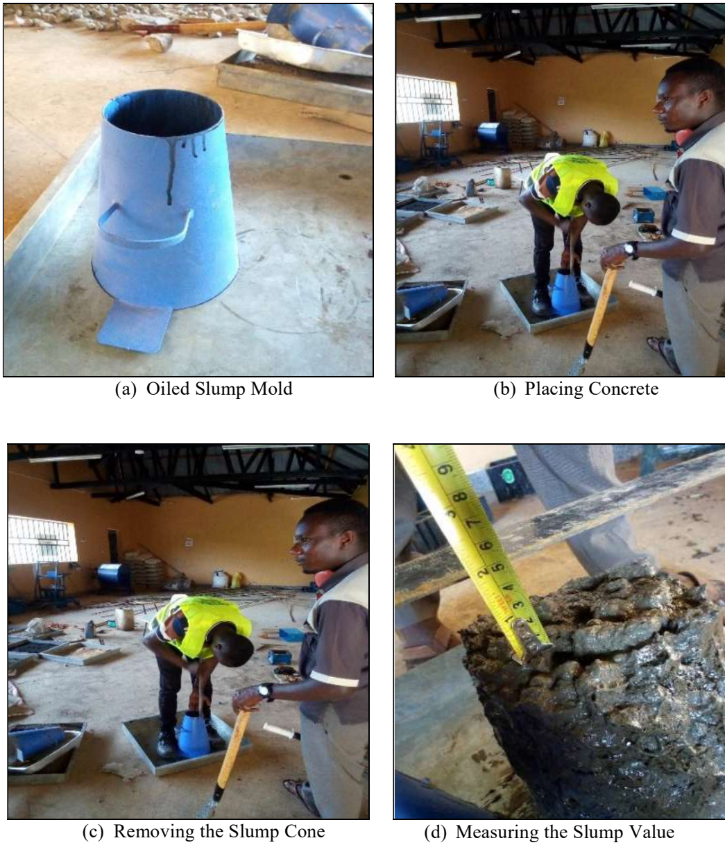
Figure 5. Procedure for Slump Test
