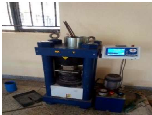
Figure 8. Concrete Specimen: Compressive Test Machine Used to Test the Compressive Strength Of Rubberized Concrete
