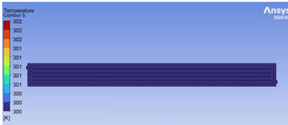
Figure 5. Heat Distribution from Effect of C-Rate on Thermal Performance for Battery with Inlet Cooling System 300K and C-rate 0.5C
