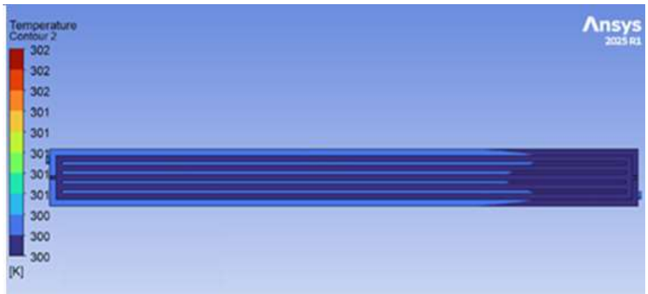
Figure 6. Heat Distribution from Effect of C-Rate on Thermal Performance for Battery with Inlet Cooling System 300K and C-rate 1C
