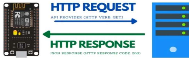
Figure 5. JSON Data Parsing Schematic
