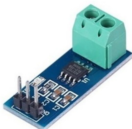
Figure 7. ACS712 Current sensor
